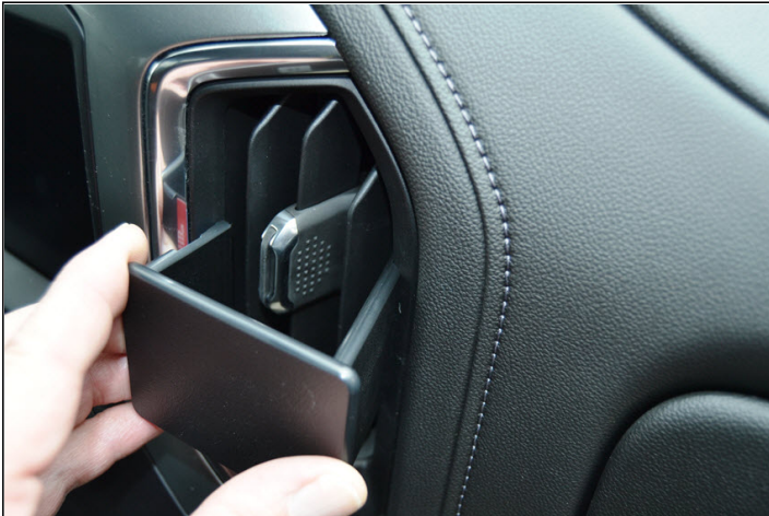
1. Clean the area where the ProClip will attach. The adhesive tape cover must be removed.
