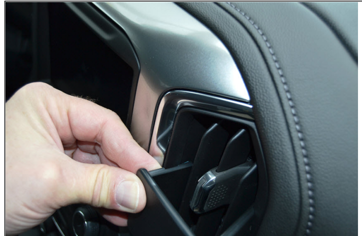
2. Press the ProClip to the right and hook the notch on the left side of the ProClip onto the left edge of the vent frame.
